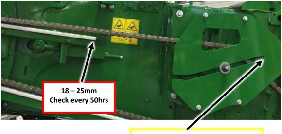
Replace chain when Idler has reached the end of adjustment slot.
