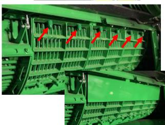
**Separator Grate Covers:** Covers a full separator grate for use in dry, high chaff conditions to improve cleaning shoe performance. Up to 2 on each side can be installed.
