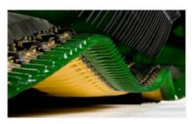
**HD:** With the wings in the down, measure 45mm at the outer reel fingers and 15mm at hinge.
