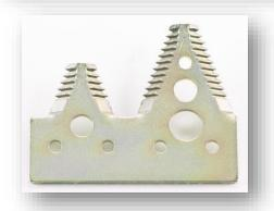
Non-Clog guards have the cross bar between the points removed to prevent stalks from plugging and a blunt nose to prevent stabbing stalks from hair pinning and pushing/plugging.
