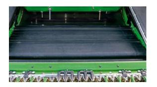
**Standard Center Belt** (RDF option only) Recommended for soybeans to promote feeding and minimize grain loss at the center section.
