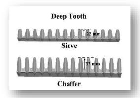
Be sure chaffer and sieve are calibrated so the opening <u>exactly</u> matches the cab display setting.
