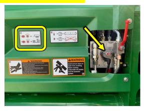
Manual Override Valve & Safety Wing Lock Ball Valve Unlocked
