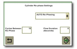
• Re-phase reminder displays a reminder to re-phase cylinders once the number of cycles is reached.
