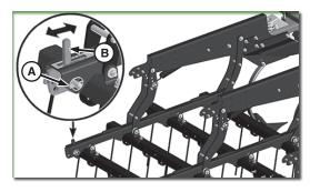
**IMPORTANT:** Make harrow tine angle adjustments with the machine raised.
