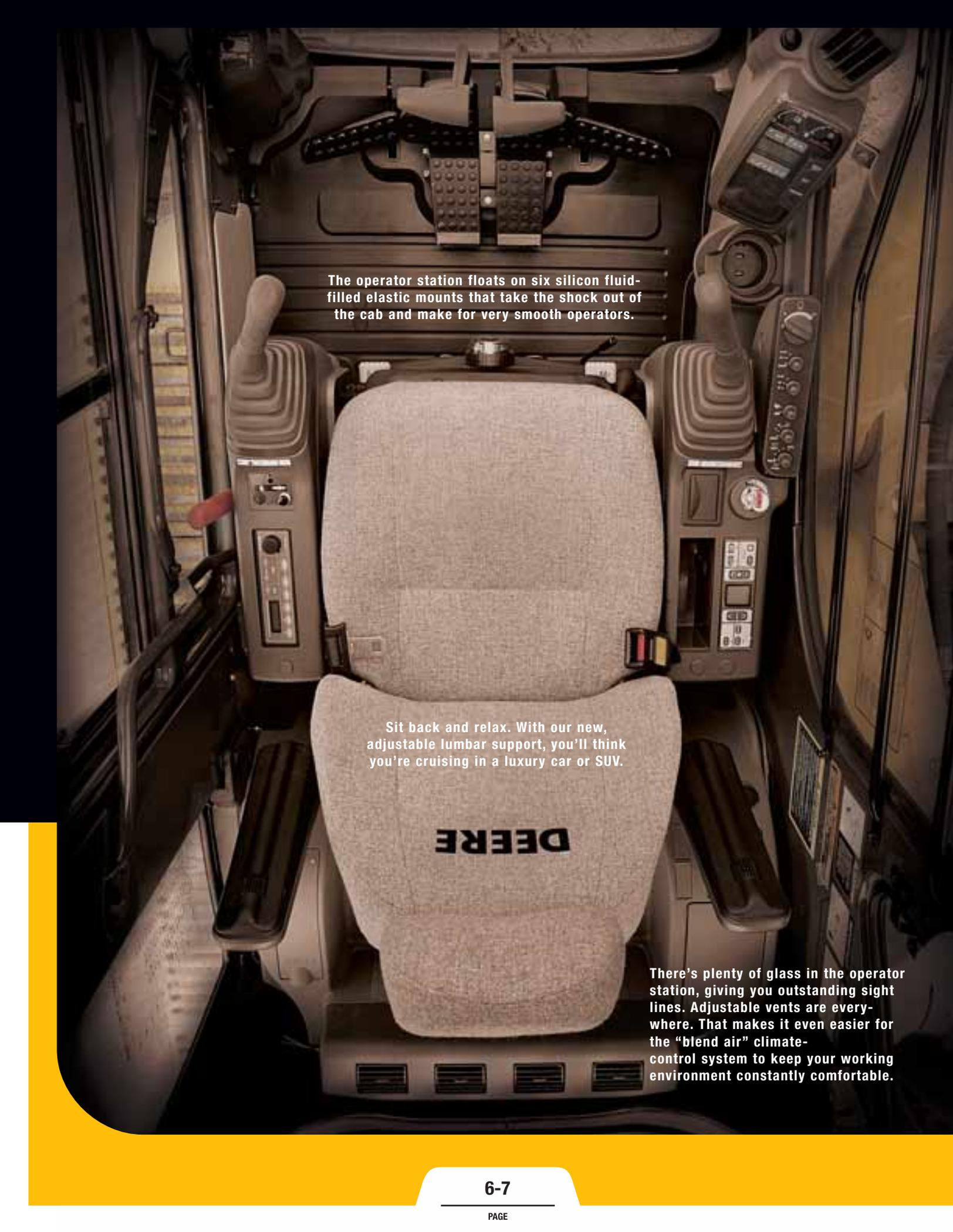
The operator station floats on six silicon fluid-filled elastic mounts that take the shock out of the cab and make for very smooth operators.
