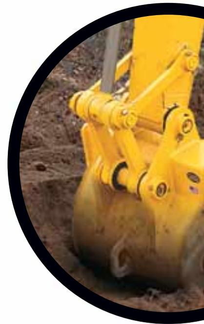
**Powdered-metal, oil-impregnated bushing in the front structure increases the greasing interval from 250 to 500 hours.**
