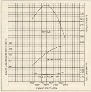
Curves shown are for an engine complete with fuel system, water pump, lubricating pump, air cleaner, alternator, fan and muffler.
