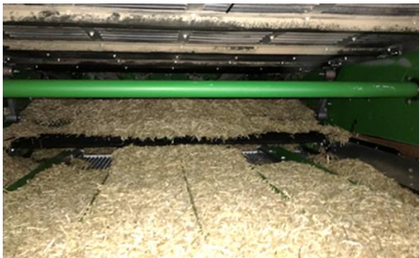
Notice chaff level is at top of dividers, in this condition, attempt to reduce chaff with less aggressive settings and/or separator
