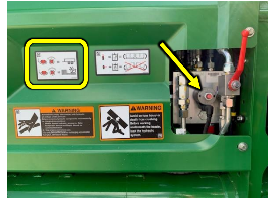
Manual Override Valve & Safety Wing Lock Ball Valve Unlocked
