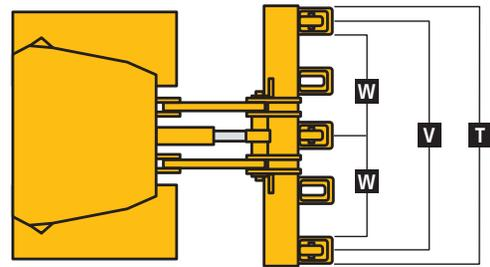
Heavy-duty parallelogram ripper, 5 shank pockets with 3 teeth
