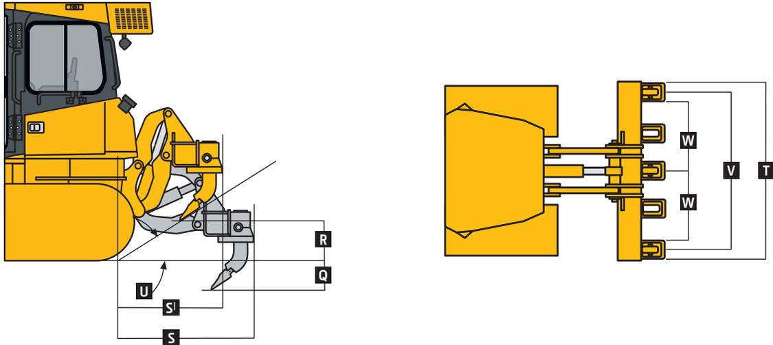
Heavy-duty parallelogram ripper, 5 shank pockets with 3 teeth
