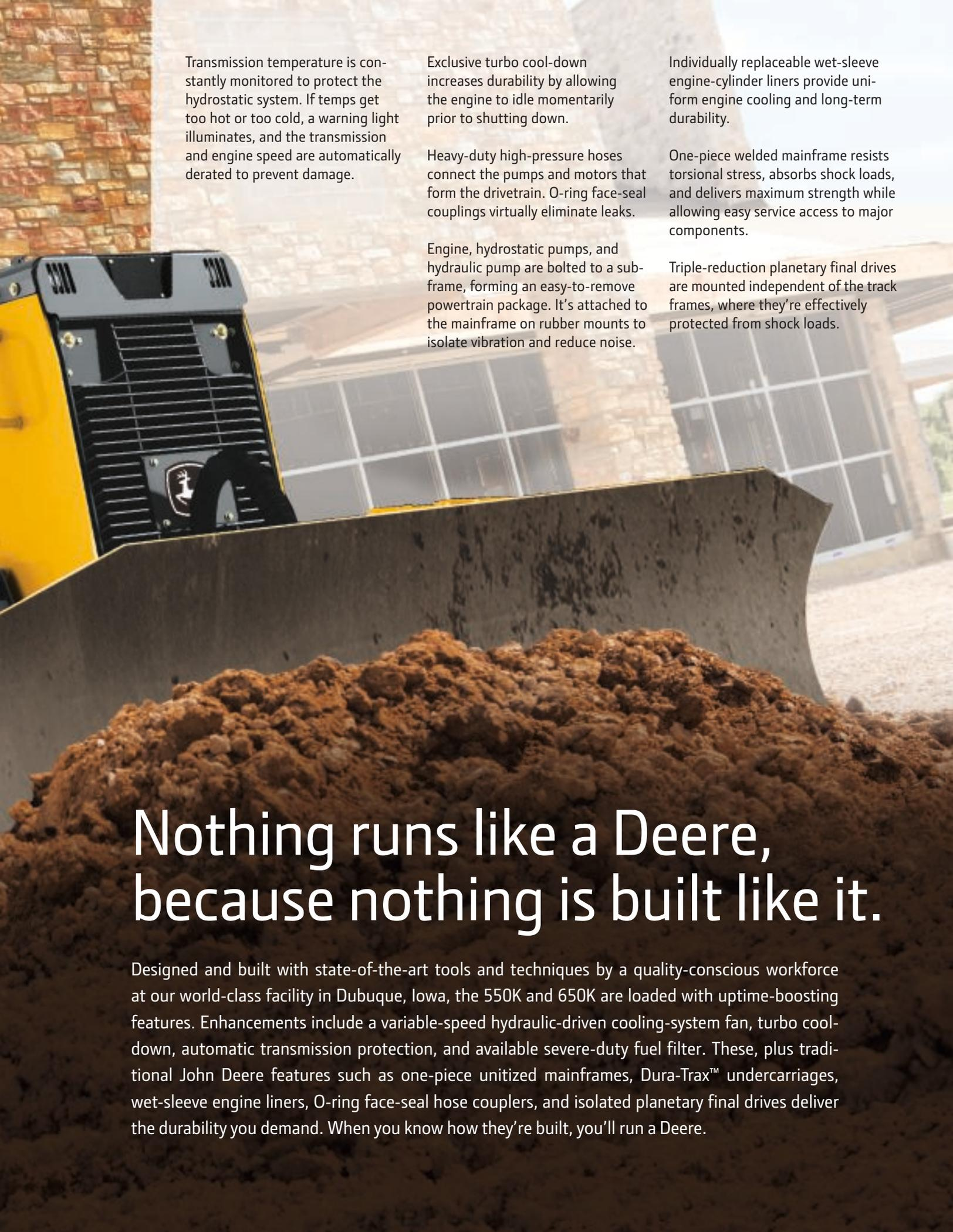
Transmission temperature is constantly monitored to protect the hydrostatic system. If temps get too hot or too cold, a warning light illuminates, and the transmission and engine speed are automatically derated to prevent damage.
